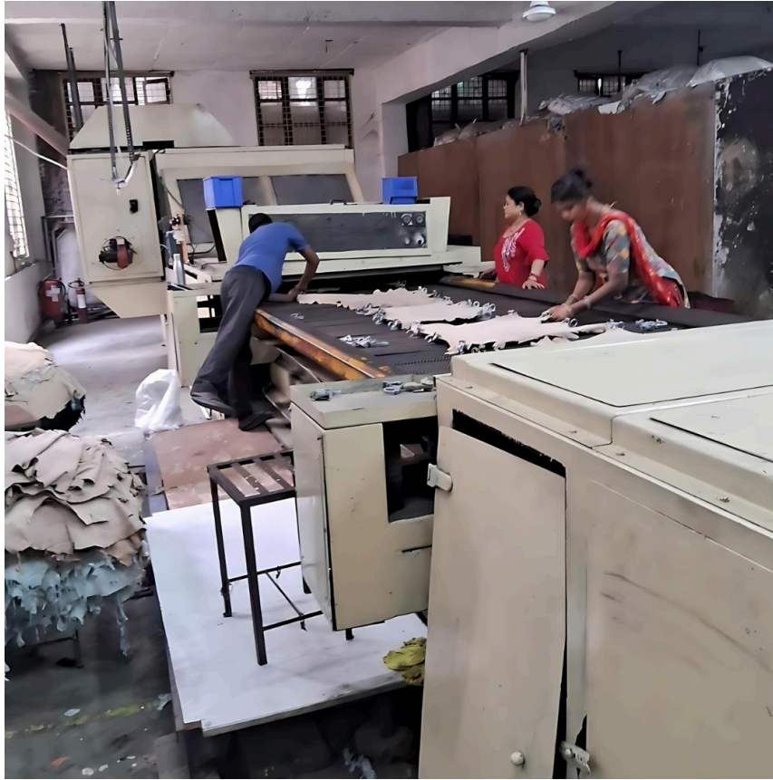
Image 2: The toggling machine with heater in close proximity to stored leather
